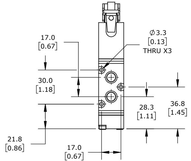
5-PORT (4-WAY), 2-POSITION, PILOT-ASSISTED ROLLER LEVER, SPRING RETURN, 1/8IN FEMALE NPT INLET(S), 1/8IN FEMALE NPT OUTLET(S), 1/8IN FEMALE NPT EXHAUST(S), CV=0.55.
