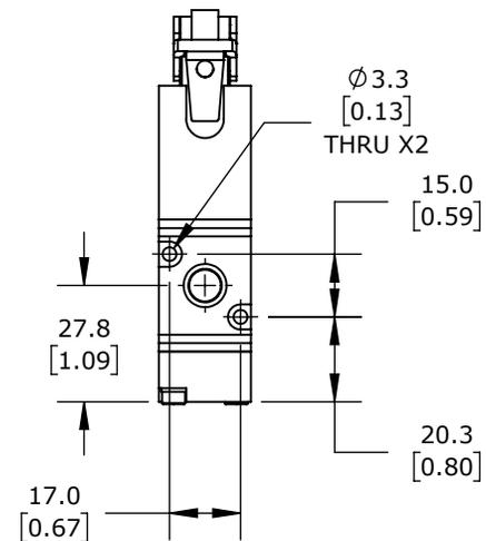
MECHANICALLY OPERATED DIRECTIONAL CONTROL VALVE, 3-PORT (3-WAY), 2-POSITION, N.C., PILOT-ASSISTED ROLLER LEVER, SPRING RETURN, 1/8IN FEMALE NPT INLET(S), 1/8IN FEMALE NPT OUTLET(S), 1/8IN FEMALE NPT EXHAUST(S), CV=0.55.
