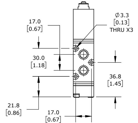
MECHANICALLY OPERATED DIRECTIONAL CONTROL VALVE, 5-PORT (4-WAY), 2-POSITION, PILOT-ASSISTED PLUNGER, SPRING RETURN, 1/8IN FEMALE NPT INLET(S), 1/8IN FEMALE NPT OUTLET(S), 1/8IN FEMALE NPT EXHAUST(S), CV=0.55.
