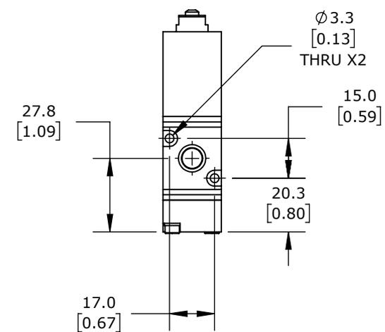
MECHANICALLY OPERATED DIRECTIONAL CONTROL VALVE, 3-PORT (3-WAY), 2-POSITION, N.C., PILOT-ASSISTED PLUNGER, SPRING RETURN, 1/8IN FEMALE NPT INLET(S), 1/8IN FEMALE NPT OUTLET(S), 1/8IN FEMALE NPT EXHAUST(S), CV=0.55.
