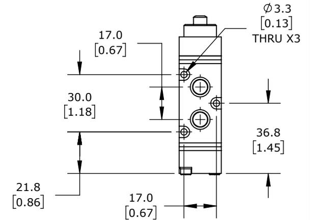
MECHANICALLY OPERATED DIRECTIONAL CONTROL VALVE, 5-PORT (4-WAY), 2-POSITION, PLUNGER, SPRING RETURN, 1/8IN FEMALE NPT INLET(S), 1/8IN FEMALE NPT OUTLET(S), 1/8IN FEMALE NPT EXHAUST(S), CV=0.55.
