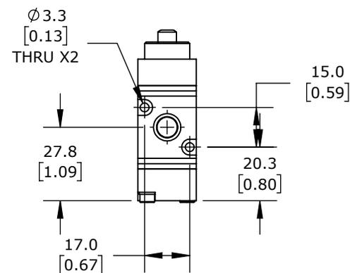
MECHANICALLY OPERATED DIRECTIONAL CONTROL VALVE, 3-PORT (3-WAY), 2-POSITION, N.C., PLUNGER, SPRING RETURN, 1/8IN FEMALE NPT INLET(S), 1/8IN FEMALE NPT OUTLET(S), 1/8IN FEMALE NPT EXHAUST(S), CV=0.55.
