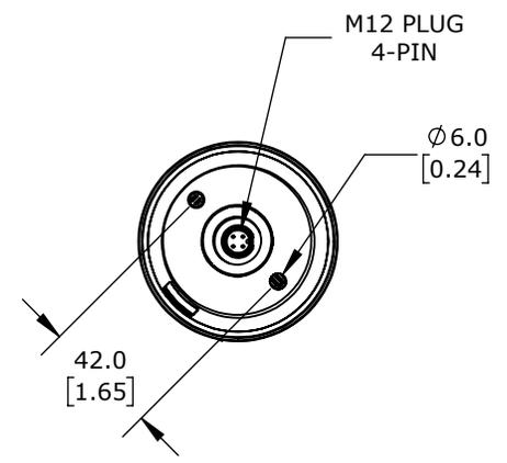
WHITE, (15) TIERS, 72MM DIAMETER, CUSTOM PROGRAMMABLE COLORS, SELECTABLE MULTI LIGHT FUNCTION, (10) SELECTABLE TONE(S), 24 VDC, 360 DEGREE VIEWING ANGLE, 4-PIN M12 A-CODED (IO-LINK), BASE OR TUBE MOUNT, IP66 AND IP69K.
