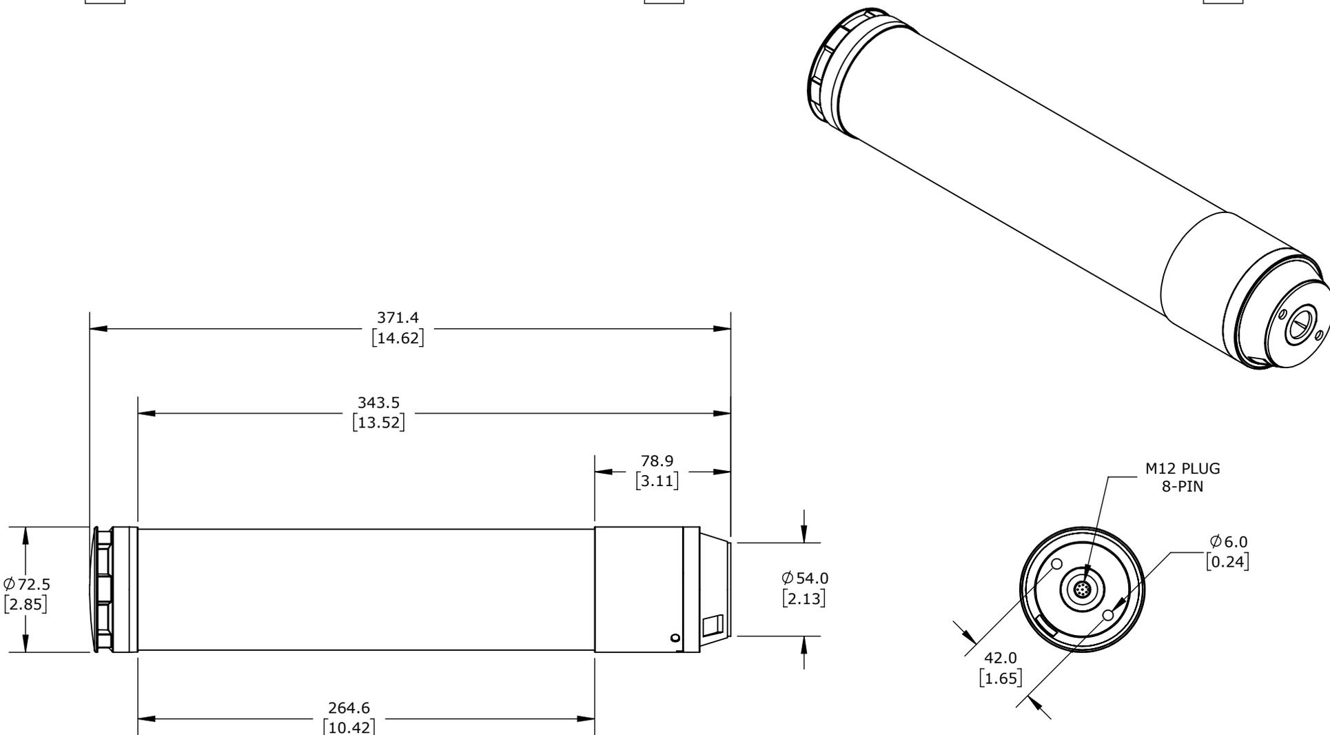
WHITE, (15) TIERS, 72MM DIAMETER, CUSTOM PROGRAMMABLE COLORS, SELECTABLE MULTI LIGHT FUNCTION, (10) SELECTABLE TONE(S), 24 VDC, 360 DEGREE VIEWING ANGLE, 8-PIN M12 A-CODED, BASE OR TUBE MOUNT, IP66 AND IP69K.
