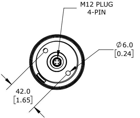
WHITE, (15) TIERS, 72MM DIAMETER, CUSTOM PROGRAMMABLE COLORS, SELECTABLE MULTI LIGHT FUNCTION, 24 VDC, 360 DEGREE VIEWING ANGLE, 4-PIN M12 A-CODED (IO-LINK), BASE OR TUBE MOUNT, IP66 AND IP69K.
