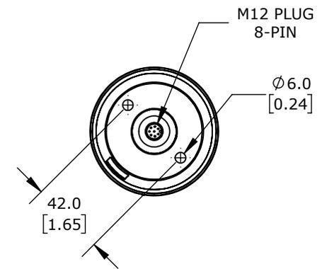
WHITE, (9) TIERS, 72MM DIAMETER, CUSTOM PROGRAMMABLE COLORS, SELECTABLE MULTI LIGHT FUNCTION, 24 VDC, 360 DEGREE VIEWING ANGLE, 8-PIN M12 A-CODED, BASE OR TUBE MOUNT, IP66 AND IP69K.
