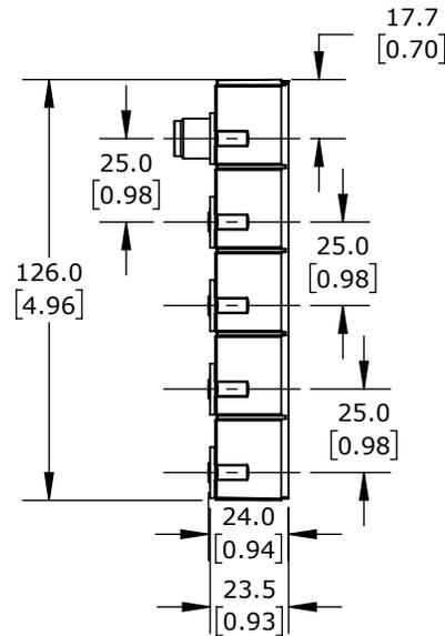
MURRELEKTRONIK IO-LINK HUB, UP TO (4) TEMPERATURE INPUT CHANNEL(s), (4) 5-PIN M12 A-CODED PORT(s), RTD, 24-BIT, IO-LINK V1.1.2 (COMPATIBLE WITH V1.1.3), IO-LINK CLASS A DEVICE, IP65, IP67 AND IP68, REQUIRES IO-LINK MASTER
