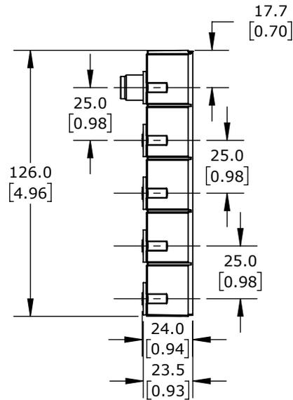
MURRELEKTRONIK IO-LINK HUB, UP TO (4) ANALOG INPUT CHANNEL(s), (4) 5-PIN M12 A-CODED PORT(s), CURRENT/VOLTAGE, 24-BIT, IO-LINK V1.1.2 (COMPATIBLE WITH V1.1.3), IO-LINK CLASS A DEVICE, IP65, IP67 AND IP68, REQUIRES IO-LINK MASTER
