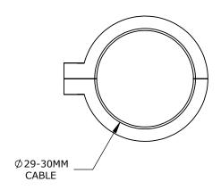
1 OPENING(S), TPE, BLACK, ACCEPTS 29-30MM DIAMETER CABLE, UL TYPE 12. PACKAGE OF 4. FOR USE WITH MURRPLASTIK KDL/D SERIES CABLE ENTRY SYSTEM FRAME.
