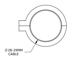
1 OPENING(S), TPE, BLACK, ACCEPTS 28-29MM DIAMETER CABLE, UL TYPE 12. PACKAGE OF 4. FOR USE WITH MURRPLASTIK KDL/D SERIES CABLE ENTRY SYSTEM FRAME.
