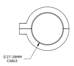
1 OPENING(S), TPE, BLACK, ACCEPTS 27-28MM DIAMETER CABLE, UL TYPE 12. PACKAGE OF 4. FOR USE WITH MURRPLASTIK KDL/D SERIES CABLE ENTRY SYSTEM FRAME.
