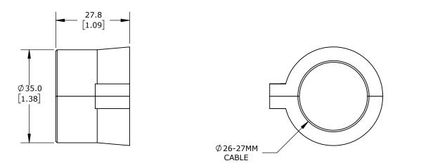
1 OPENING(S), TPE, BLACK, ACCEPTS 26-27MM DIAMETER CABLE, UL TYPE 12. PACKAGE OF 4. FOR USE WITH MURRPLASTIK KDL/D SERIES CABLE ENTRY SYSTEM FRAME.
