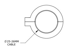
1 OPENING(S), TPE, BLACK, ACCEPTS 25-26MM DIAMETER CABLE, UL TYPE 12. PACKAGE OF 4. FOR USE WITH MURRPLASTIK KDL/D SERIES CABLE ENTRY SYSTEM FRAME.
