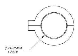
1 OPENING(S), TPE, BLACK, ACCEPTS 24-25MM DIAMETER CABLE, UL TYPE 12. PACKAGE OF 4. FOR USE WITH MURRPLASTIK KDL/D SERIES CABLE ENTRY SYSTEM FRAME.
