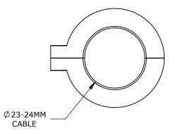
1 OPENING(S), TPE, BLACK, ACCEPTS 23-24MM DIAMETER CABLE, UL TYPE 12. PACKAGE OF 4. FOR USE WITH MURRPLASTIK KDL/D SERIES CABLE ENTRY SYSTEM FRAME.
