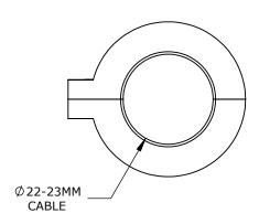
1 OPENING(S), TPE, BLACK, ACCEPTS 22-23MM DIAMETER CABLE, UL TYPE 12. PACKAGE OF 4. FOR USE WITH MURRPLASTIK KDL/D SERIES CABLE ENTRY SYSTEM FRAME.
