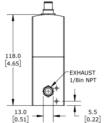
METAL WORK REGTRONIC PNEUMATIC TRANSDUCER, 4-20 mA, 0-5 VDC OR 0-10 VDC INPUT, 0.05-10 bar ADJUSTABLE OUTPUT PRESSURE, 4-20 mA, SWITCH (N.O./N.C.) PNP/NPN OUTPUT, 1/8in FEMALE NPT INLET(S), 1/8in FEMALE NPT OUTLET(S), 8-PIN M12 QUICK-DISCONNECT, IP65
