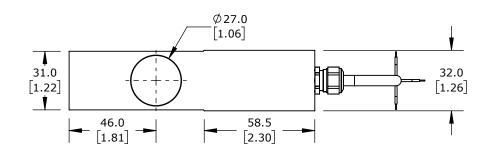
SENSY BENDING BEAM LOAD CELL, 3306 LB/1500 KG, +/- 0.3% OF FULL SCALE ACCURACY, VOLTAGE SIGNAL RANGE(s) OF 1.8-2.2 MV/V, 3-12 VDC, STAINLESS STEEL, IP67, 26.2FT/8M INTEGRAL 4-WIRE SHIELDED CABLE
