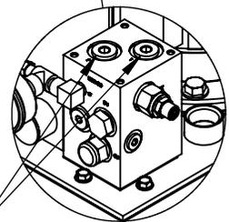
SAE O-RING BOSS (ORB) #6 P / T HYDRAULIC CONNECTION
