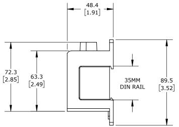
FINGER-SAFE, 85A, 1-POLE, LINE SIDE: 1 OPENING ACCEPTS 3 AWG TO 14 AWG, LOAD SIDE: 6 OPENINGS ACCEPT 8 AWG TO 14 AWG, PANEL OR 35MM DIN RAIL MOUNT, UL 1953 LISTED.
