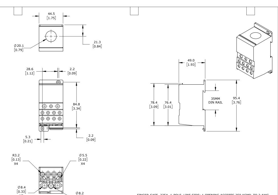
FINGER-SAFE, 225A, 1-POLE, LINE SIDE: 1 OPENING ACCEPTS 250 KCMIL TO 2 AWG, LOAD SIDE: 2 OPENINGS ACCEPT 2 AWG TO 14 AWG & 5 OPENINGS ACCEPT 6 AWG TO 14 AWG & 4 OPENINGS ACCEPT 8 AWG TO 14 AWG, PANEL OR 35MM DIN RAIL MOUNT.
