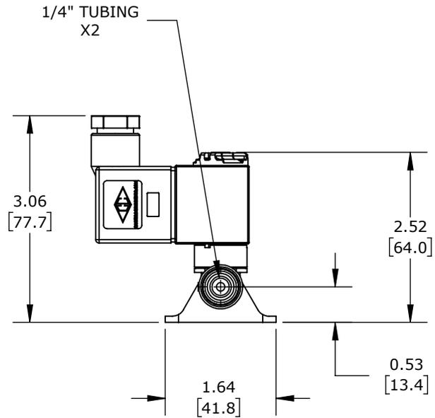
2-WAY, 2-POSITION, N.C., ACETAL BODY, 1/4IN PUSH-TO-CONNECT TUBING INLET(s), 1/4IN PUSH-TO-CONNECT TUBING OUTLET(s), CV=0.24, 150 PSI MAXIMUM OPERATING PRESSURE, 120 VAC OPERATING VOLTAGE, 11mm DIN STYLE WIRING PLUG.
