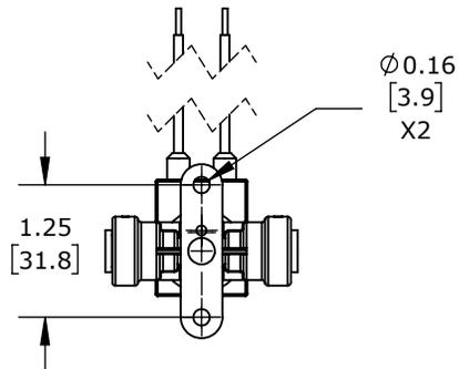
2-WAY, 2-POSITION, N.C., ACETAL BODY, 1/4IN PUSH-TO-CONNECT TUBING INLET(s), 1/4IN PUSH-TO-CONNECT TUBING
