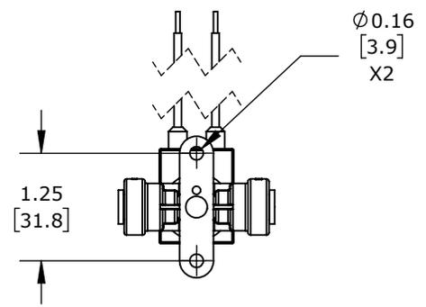
2-WAY, 2-POSITION, N.C., ACETAL BODY, 1/4IN PUSH-TO-CONNECT TUBING INLET(s), 1/4IN PUSH-TO-CONNECT TUBING OUTLET(s), CV=0.24, 150 PSI MAXIMUM OPERATING PRESSURE, 24 VDC OPERATING VOLTAGE, 18IN PIGTAIL.
