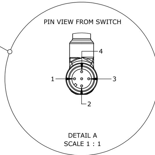
IDEM PUSHBUTTON, IP65, 22MM, MOMENTARY, (1) N.O./ (1) N.C. CONTACT(S), BLACK, MUSHROOM, 68MM, ROUND. FOR USE WITH IDEM TWO-HAND SAFETY CONTROL PANELS.
