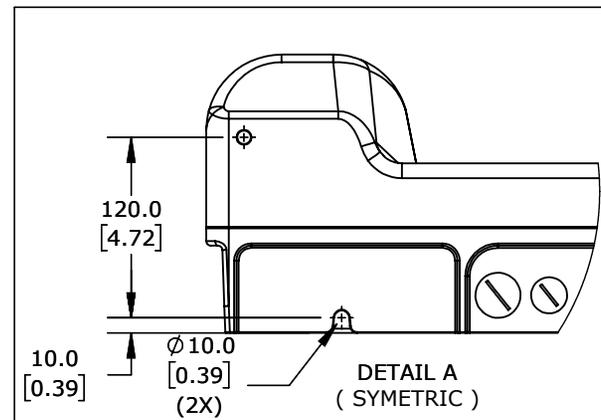
IDEM CONTROL PANEL, TWO-HAND SAFETY, DIE-CAST ALUMINUM, EMPTY ENCLOSURE.
