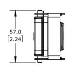
DOUBLE LEVER, CONNECTOR HOUSING SIZE 16B, HEAVY-DUTY THERMOPLASTIC. FOR USE WITH METE SIZE 16B 4-PEG CONNECTOR HOUSINGS.
