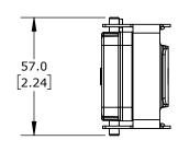
DOUBLE LEVER, CONNECTOR HOUSING SIZE 10B, HEAVY-DUTY THERMOPLASTIC. FOR USE WITH METE SIZE 10B 4-PEG CONNECTOR HOUSINGS.
