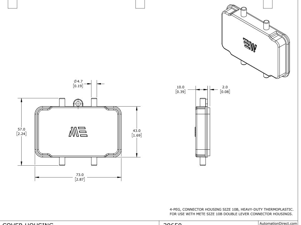
METE COVER HOUSING 29650 1-800-633-0405 3rd PART DIMENSIONS MAY DIFFER SLIGHTLY METRIC UNITS USED UNLESS OTHERWISE LATEST VERSION NOT TO mm SHEET 1 OF 1 ANGLE SPECIFIED UNITS ARE: [inch] SCALE FOR PART DESIGN 2/12/2025 DUE TO MANUFACTURER'S VARIANCES
