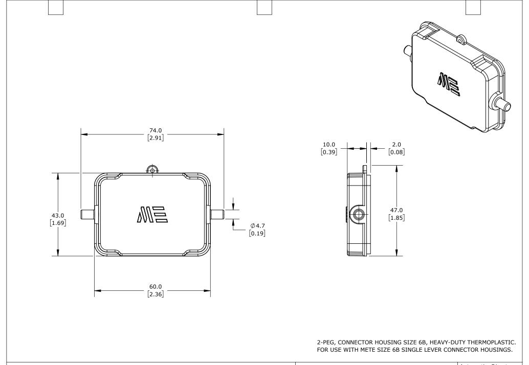
AutomationDirect.com METE COVER HOUSING 29644 1-800-633-0405 3rd PART DIMENSIONS MAY DIFFER SLIGHTLY METRIC UNITS USED UNLESS OTHERWISE LATEST VERSION NOT TO mm SHEET 1 OF 1 ANGLE SPECIFIED UNITS ARE: [inch] SCALE FOR PART DESIGN 2/12/2025 DUE TO MANUFACTURER'S VARIANCES
