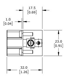
CONNECTOR HOUSING SIZE 16A, 16-POLE, SCREW TERMINALS, ACCEPTS WIRE SIZE 18-14 AWG, 16 AMP, 600 VAC/VDC, POLES NUMBERED 1 TO 16. FOR USE WITH METE MULTI-WIRE HOUSINGS.
