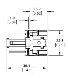
CONNECTOR HOUSING SIZE 16A, 25-POLE, CRIMPED CONTACT, 10 AMP, 600 VAC/VDC, POLES NUMBERED 1 TO 25. FOR USE WITH METE MULTI-WIRE HOUSINGS. REQUIRES 10 AMP FEMALE CONTACTS METE 14103XXX.
