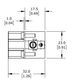
CONNECTOR HOUSING SIZE 10A, 10-POLE, SCREW TERMINALS, ACCEPTS WIRE SIZE 18-14 AWG, 16 AMP, 600 VAC/VDC, POLES NUMBERED 1 TO 10. FOR USE WITH METE MULTI-WIRE HOUSINGS.
