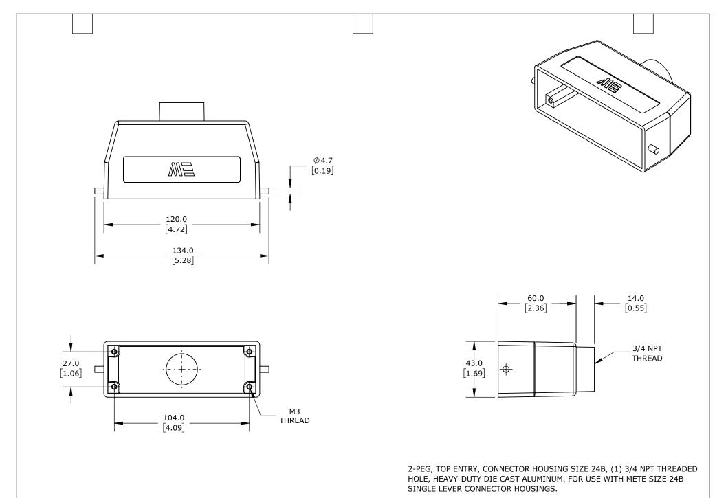
AutomationDirect.com METE HOOD HOUSING 293742905 1-800-633-0405 UNLESS OTHERWISE NOT TO PART DIMENSIONS MAY DIFFER SLIGHTLY METRIC UNITS USED LATEST VERSION 3rd mm SHEET 1 OF 1 ANGLE SCALE FOR PART DESIGN SPECIFIED UNITS ARE: [inch] DUE TO MANUFACTURER'S VARIANCES 2/12/2025
