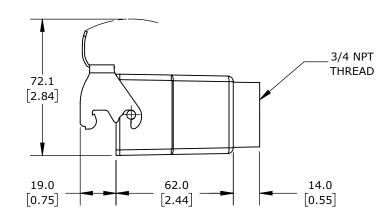
SINGLE LEVER, TOP ENTRY, CONNECTOR HOUSING SIZE 16B, (1) 3/4 NPT THREADED HOLE, HEAVY-DUTY DIE CAST ALUMINUM. FOR USE WITH METE SIZE 16B 2-PEG CONNECTOR HOUSINGS.
