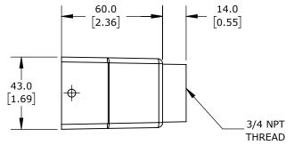
2-PEG, TOP ENTRY, CONNECTOR HOUSING SIZE 16B, (1) 3/4 NPT THREADED HOLE, HEAVY-DUTY DIE CAST ALUMINUM. FOR USE WITH METE SIZE 16B SINGLE LEVER CONNECTOR HOUSINGS.
