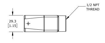
2-PEG, TOP ENTRY, CONNECTOR HOUSING SIZE 16A, (1) 1/2 NPT THREADED HOLE, HEAVY-DUTY DIE CAST ALUMINUM. FOR USE WITH METE SIZE 16A SINGLE LEVER CONNECTOR HOUSINGS.
