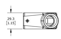
2-PEG, SIDE ENTRY, CONNECTOR HOUSING SIZE 16A, (1) 1/2 NPT THREADED HOLE, HEAVY-DUTY DIE CAST ALUMINUM. FOR USE WITH METE SIZE 16A SINGLE LEVER CONNECTOR HOUSINGS.
