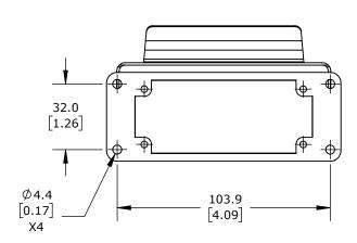
SINGLE LEVER, CONNECTOR HOUSING SIZE 16B, HEAVY-DUTY DIE CAST ALUMINUM. FOR USE WITH METE SIZE 16B 2-PEG CONNECTOR HOUSINGS.
