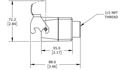
SINGLE LEVER, TOP ENTRY, CONNECTOR HOUSING SIZE 10B, (1) 1/2 NPT THREADED HOLE, HEAVY-DUTY DIE CAST ALUMINUM. FOR USE WITH METE SIZE 10B 2-PEG CONNECTOR HOUSINGS.
