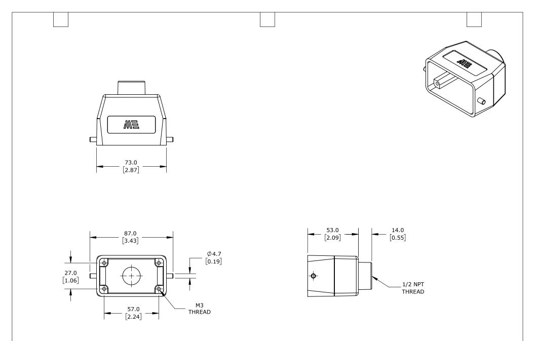
2-PEG, TOP ENTRY, CONNECTOR HOUSING SIZE 10B, (1) 1/2 NPT THREADED HOLE, HEAVY-DUTY DIE CAST ALUMINUM. FOR USE WITH METE SIZE 10B SINGLE LEVER CONNECTOR HOUSINGS.
