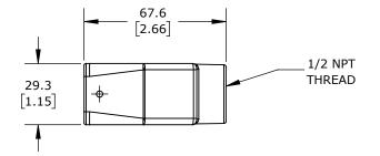
2-PEG, TOP ENTRY, CONNECTOR HOUSING SIZE 10A, (1) 1/2 NPT THREADED HOLE, HEAVY-DUTY DIE CAST ALUMINUM. FOR USE WITH METE SIZE 10A SINGLE LEVER CONNECTOR HOUSINGS.
