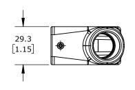
2-PEG, SIDE ENTRY, CONNECTOR HOUSING SIZE 10A, (1) 1/2 NPT THREADED HOLE, HEAVY-DUTY DIE CAST ALUMINUM. FOR USE WITH METE SIZE 10A SINGLE LEVER CONNECTOR HOUSINGS.
