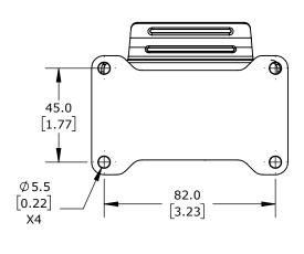
SINGLE LEVER, SIDE ENTRY, CONNECTOR HOUSING SIZE 10B, (1) 1/2 NPT THREADED HOLE, HEAVY-DUTY DIE CAST ALUMINUM. FOR USE WITH METE SIZE 10B 2-PEG CONNECTOR HOUSINGS.
