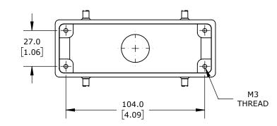
> 4-PEG, TOP ENTRY, CONNECTOR HOUSING SIZE 24B, (1) 3/4 NPT THREADED HOLE, HEAVY-DUTY DIE CAST ALUMINUM. FOR USE WITH METE SIZE 24B DOUBLE LEVER CONNECTOR HOUSINGS.
