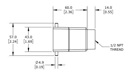
4-PEG, TOP ENTRY, CONNECTOR HOUSING SIZE 16B, (1) 1/2 NPT THREADED HOLE, HEAVY-DUTY DIE CAST ALUMINUM. FOR USE WITH METE SIZE 16B DOUBLE LEVER CONNECTOR HOUSINGS.
